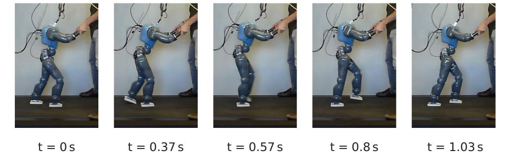
The gait controller is optimized in a **simulation environment**. The objective function rewards solutions minimizing the **metabolic energy** consumption.
